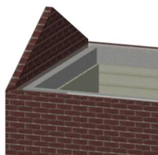
The overall thickness of a wall is equal to the sum of its components. Component fill and pen style are only displayed in Top/Plan view (except for section viewports in the Vectorworks Design Series products).
