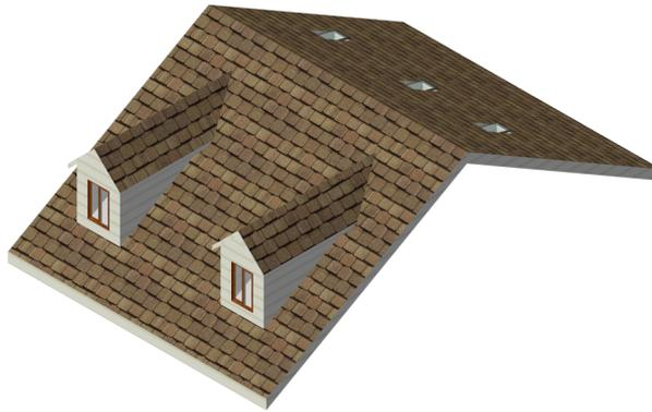
You can create a wide variety of dormer windows in roof objects and roof faces. There are five styles to select from: trapezium, gable, shed, hip, and bat; each gable type has unique parameters. The editing parameters available in the Edit Roof Element dialog box depend on the style of dormer chosen.
