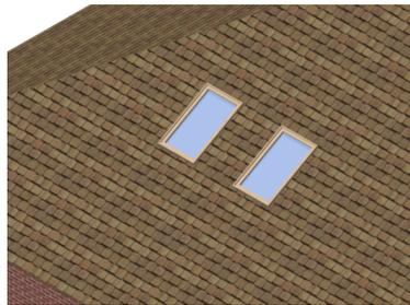
A full skylight, complete with a window symbol, can be placed in the roof object or roof face.
